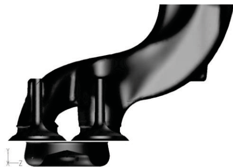
Figure 1: View of the inlet duct with two inlet valves and the piston bowl (Deutz).
