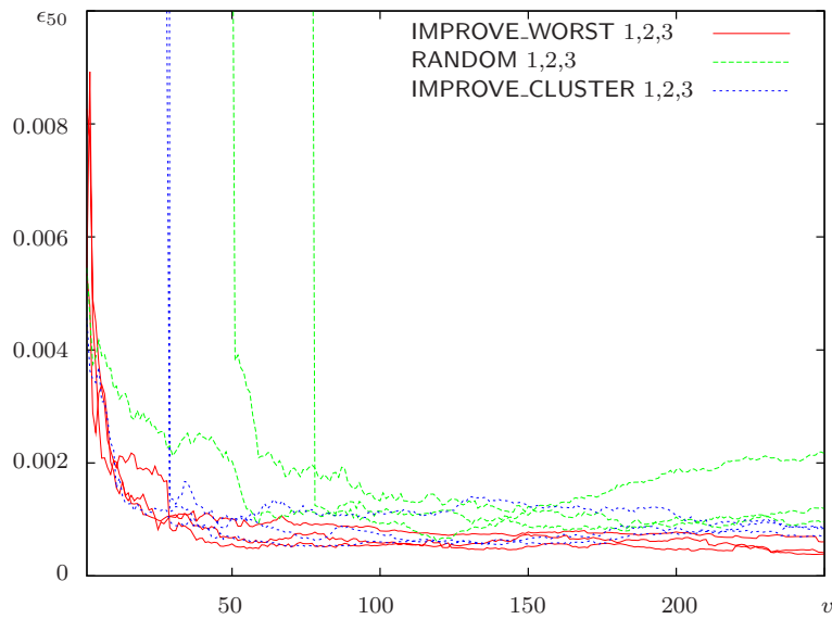
(b) Evaluation of median 3D errors \epsilon_{50} in meters. View planning using strategy IMPROVE_CLUSTER performs better than RANDOM.
