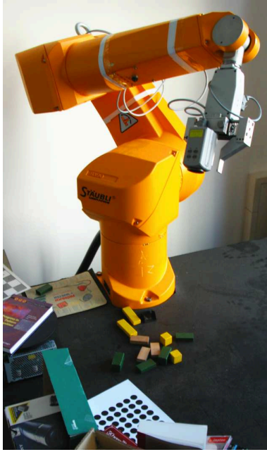
Figure 1.1: An intensity camera mounted on a robotic arm serving as controlled environment.
