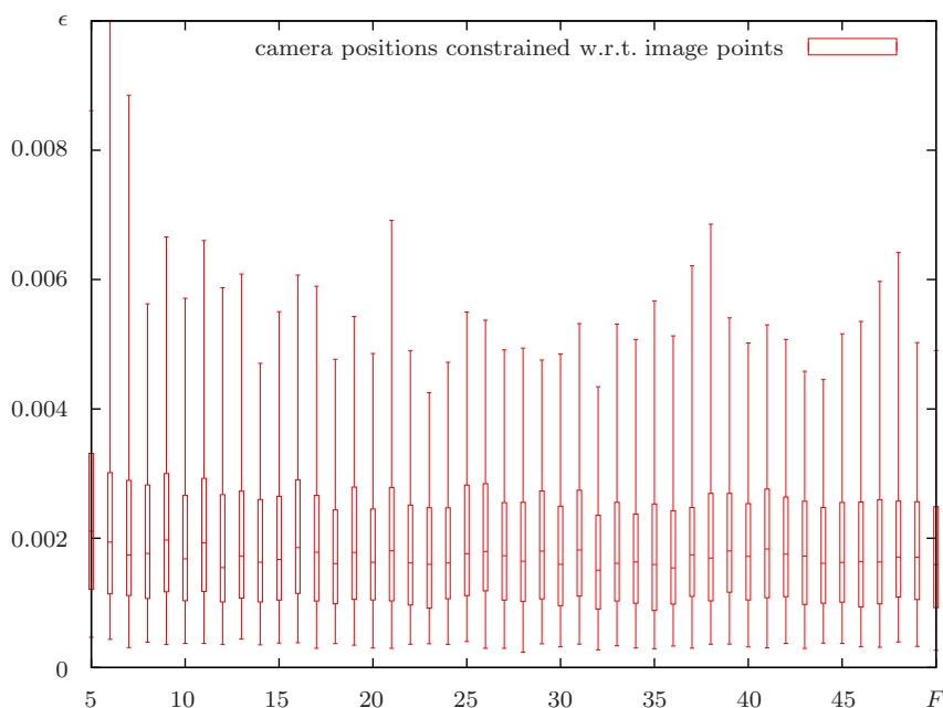
Figure 6.23: Reconstruction errors for P = 5 random points and F = 5, 6, \dots, 50 camera positions that are random but optimized towards a maximal ratio of the singular values of the image points, i. e. preferably collinear image points in the respective image.
