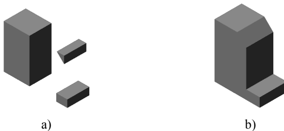
Fig. 7 Constructive solid geometry: a) basic objects b) result model
