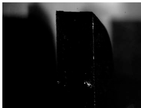
Fig. 8: Snapshot of saw tooth with cutting edges, captured in transmitted lighting mode (track speed = 10 m/min, GFE)
