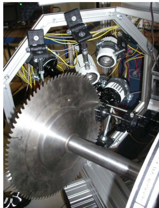
Fig. 6: Test setup with circular saw on rotating spindle, lighting, and the trigger unit
