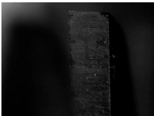
Fig. 7: Snapshot of saw tooth cutting edges and wear (track speed = 10 m/min, GFE)
