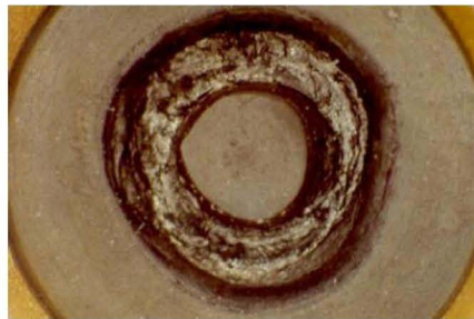
Fig. 9. Seal damage due to the surface fatigue.
