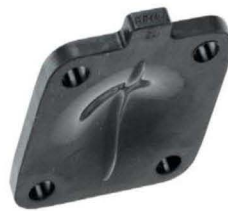
Fig. 6. Result of abrasive wear.
