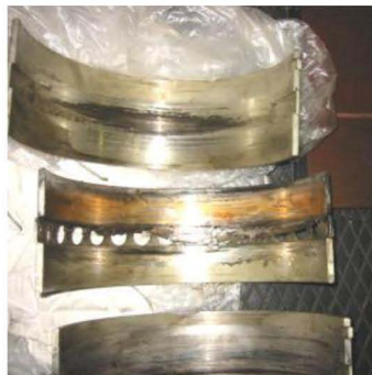
Fig. 2. Damaged engine bearings due to adhesion
