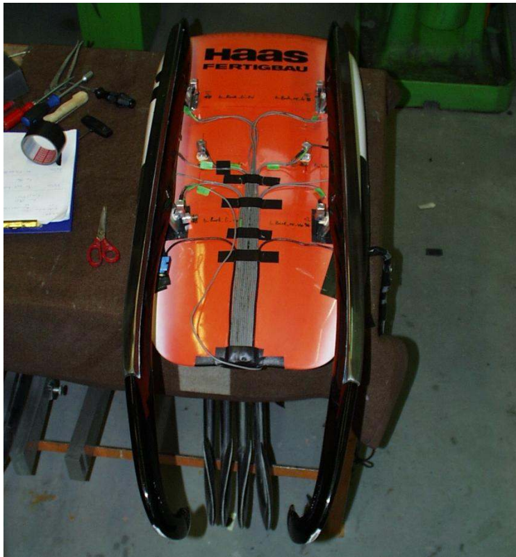
Figure 2: Luge with acceleration sensors
