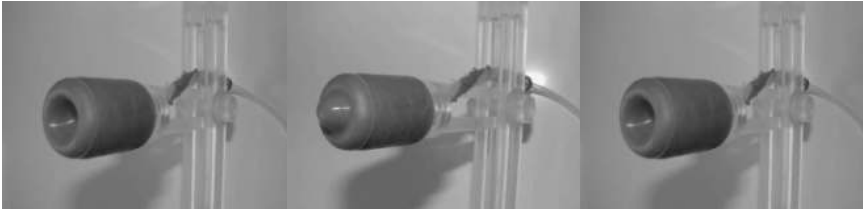
Fig 12: Snap-Through Body with Hyperelastic Material Properties. 1 Initial State without Inner Pressure, 2 Under Pressure Load 3 After Decreasing the Load
