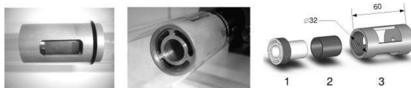
Fig. 11: Integrated Closing Device. The snap-through body of silicone is fixed on part 1. The part 1 is inserted in part 3 and can adjust with a thread.
