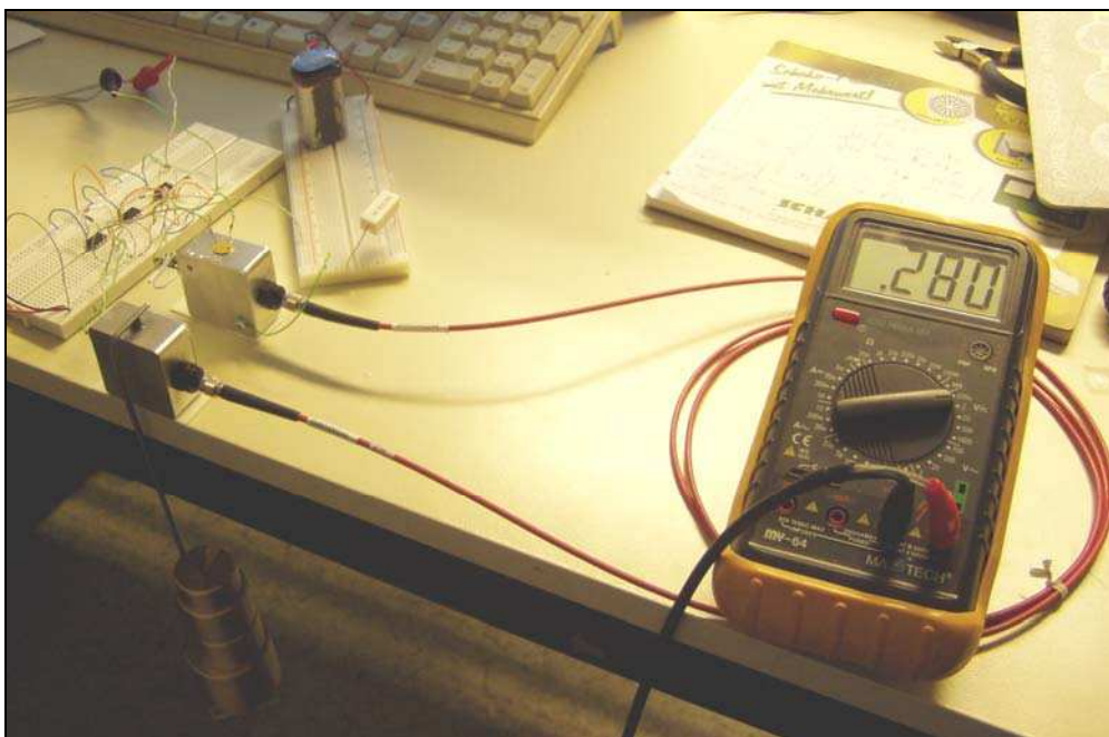
Fig. 6, Verification of the force sensor with calibrated masses.
