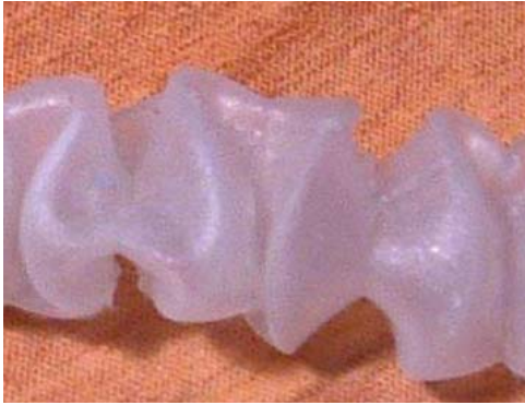
Fig.8. Structural instability of test object for vacuum
