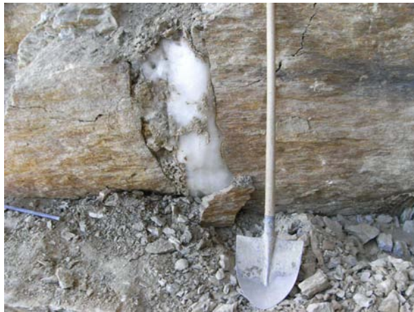
Fig. 3.9: Ice-filled crack observed close to the monitoring profile at the Stockhorn plateau (Photo: M. Baum 2007).
