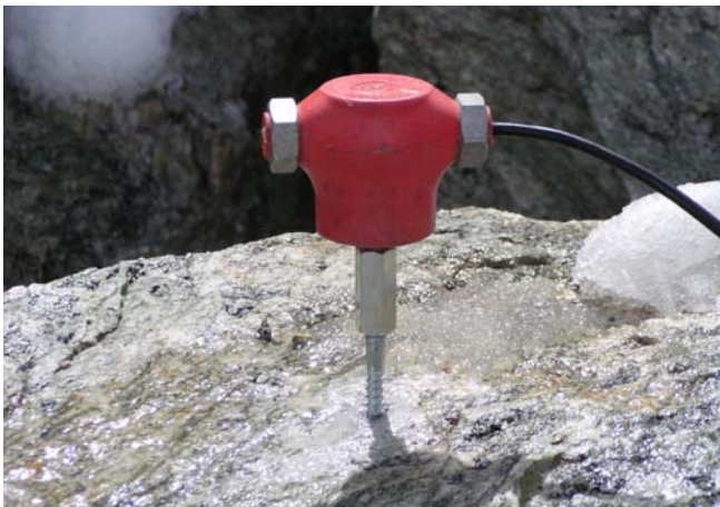
Fig. 2.6: Example of a geophone mounted on a fixed screw to a large block.
