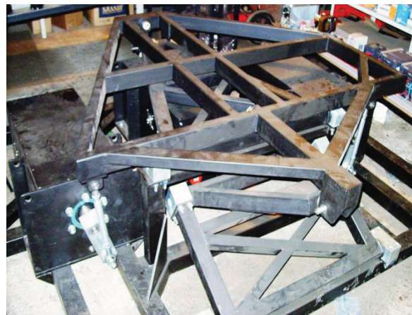
Figure 1 3-DOF movement simulator
