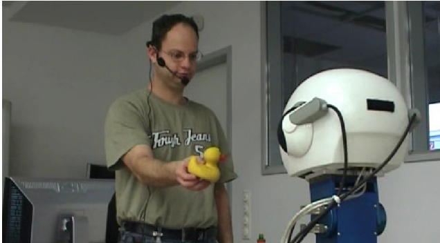
Figure 1.2: Interactive Learning of Visual Representations. The interactive learning of different visual representations is based on complex-shaped and hand-held objects presented in the near range of an active vision system. Furthermore the corresponding class hypothesis of the current presented object is communicated based on speech phrases, while a human tutor can confirm or correct this hypothesis based on the integration of a speech recognition system into a state-based user interface.
