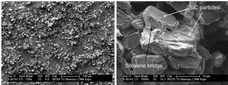
Figure 2 SEM Images of SiC particles after deposition (600°C). A smaller agglomeration because of the particle size and the Siloxane bonding bridges can be obtained.
