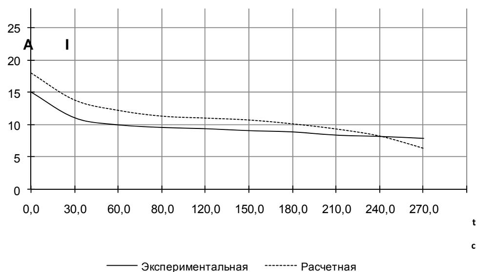
Figure 1. Current curves of the accumulator cell breakdown through fixed
