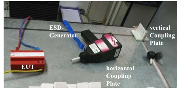
Figure 7 – Test Setup for ESD-tests
