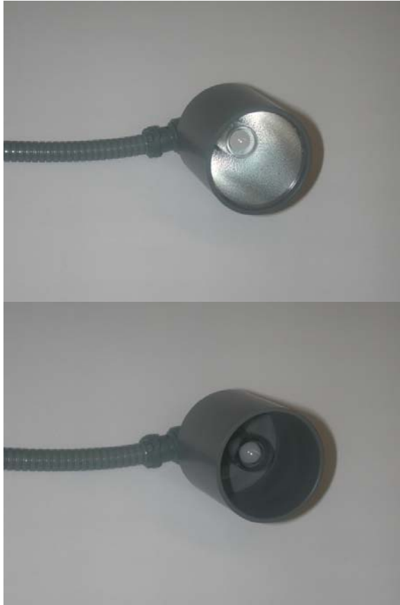
Figure 10: Optimized optical sensor with reflector shield (above: with inner reflection layer, below: without inner reflection layer)
