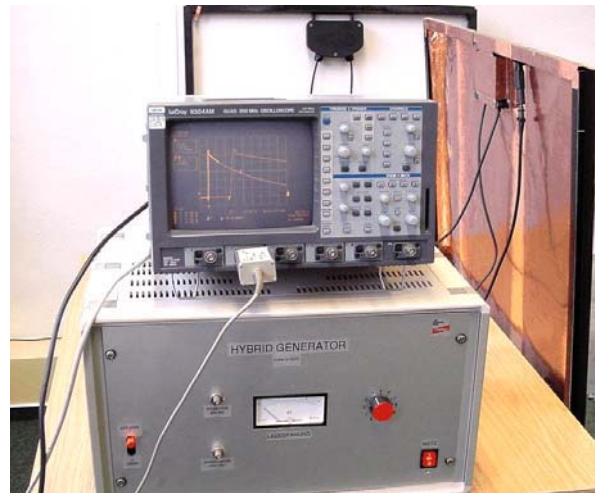
Figure 6 – Impulse voltage test
