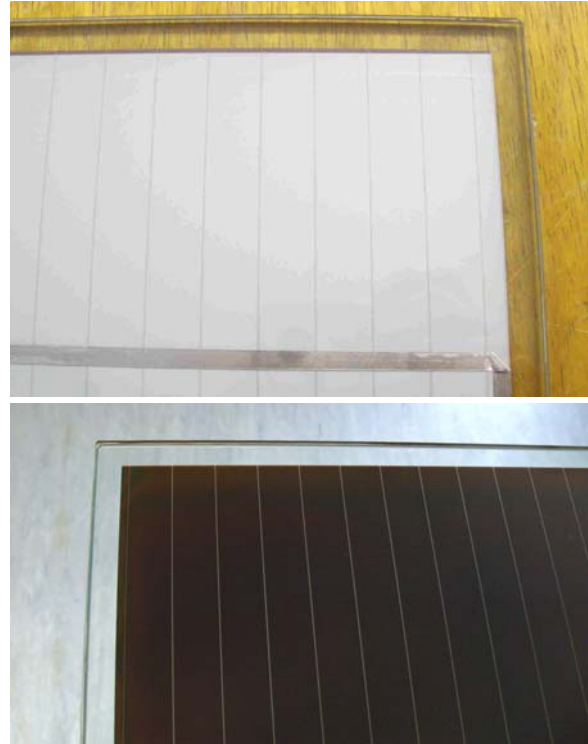
Figure 1 – Polycrystalline silicon photovoltaic module in frame construction and a frameless thin film module
