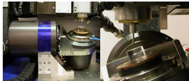
Fig. 2 Close-up view shows a PMMA substrate mounted on the thermo chuck, a diamond-microcutter as well as the lubrication system.
