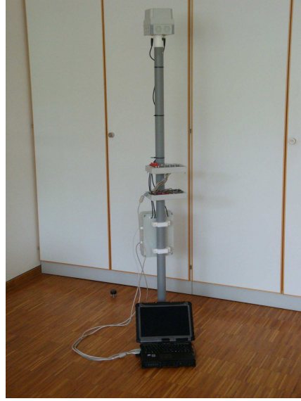
Figure 6 shows the experimental setup. At the top there is the 3D ferrite antenna, then follows the unit containing the electronic compass, the pressure sensor and the local display. In the box on the rear side there are the PicoScope, type 3424 and the antenna amplifiers connected to the laptop at the bottom.
