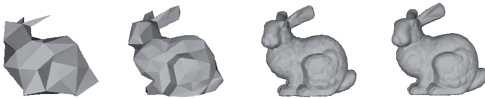
Fig. 5.21: Graphical example for the concept of dynamic level of detail (LOD). The LOD is increased for objects closer to the viewer, such that more details are visible (or audible in the equivalent acoustical case) when approaching the object (from left to right). The Stanford Bunny model from the Stanford 3D Scanning Repository [w-sta].
