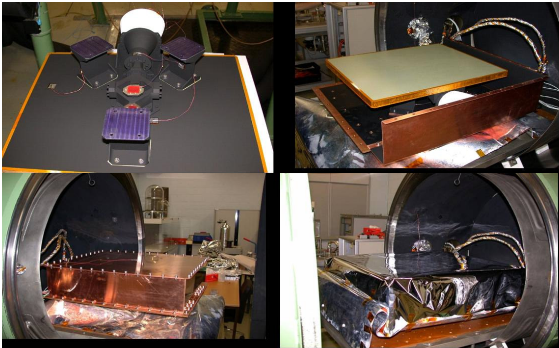
Figure 10 Thermal cycling test set-up at Astrium Ottobrunn thermal test facility
