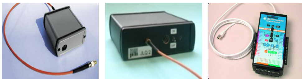
(a) Mikrospektrometer NIR 1.7 [10] (b) Lichtquelle JLQ 2 NIR [47] (c) A/D-Wandler DT9802 [22]
