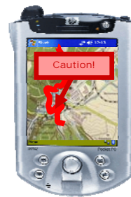
Figure 5: Mobile user terminal(PDA) with installed route planning software and visual and tactile notification of an obstacle
