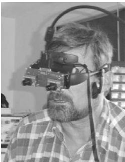
Figure 4: Visual aid system BIELORIS (Parthier2005) helps to increase the edge detection ability of high-grade visual impaired based on Sobel-algorithms
