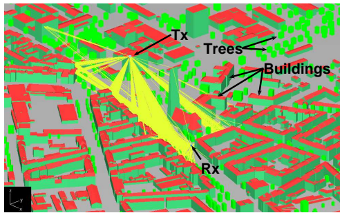
(a) 3D environment of Karlsruhe city showing the paths calculated by the raytracer
