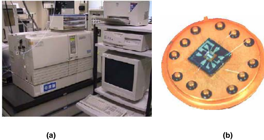
Fig. 1: (a) Standard analytical instrument (chromatography/mass spectrometry). (b) Semiconductor based gas sensor.
