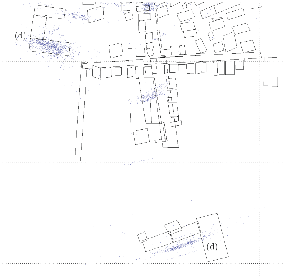
Fig. 5.74: Magnified view of the far scatterers from Figure 5.72. The buildings marked with (d) are particularly well resolved by the localization algorithm.
