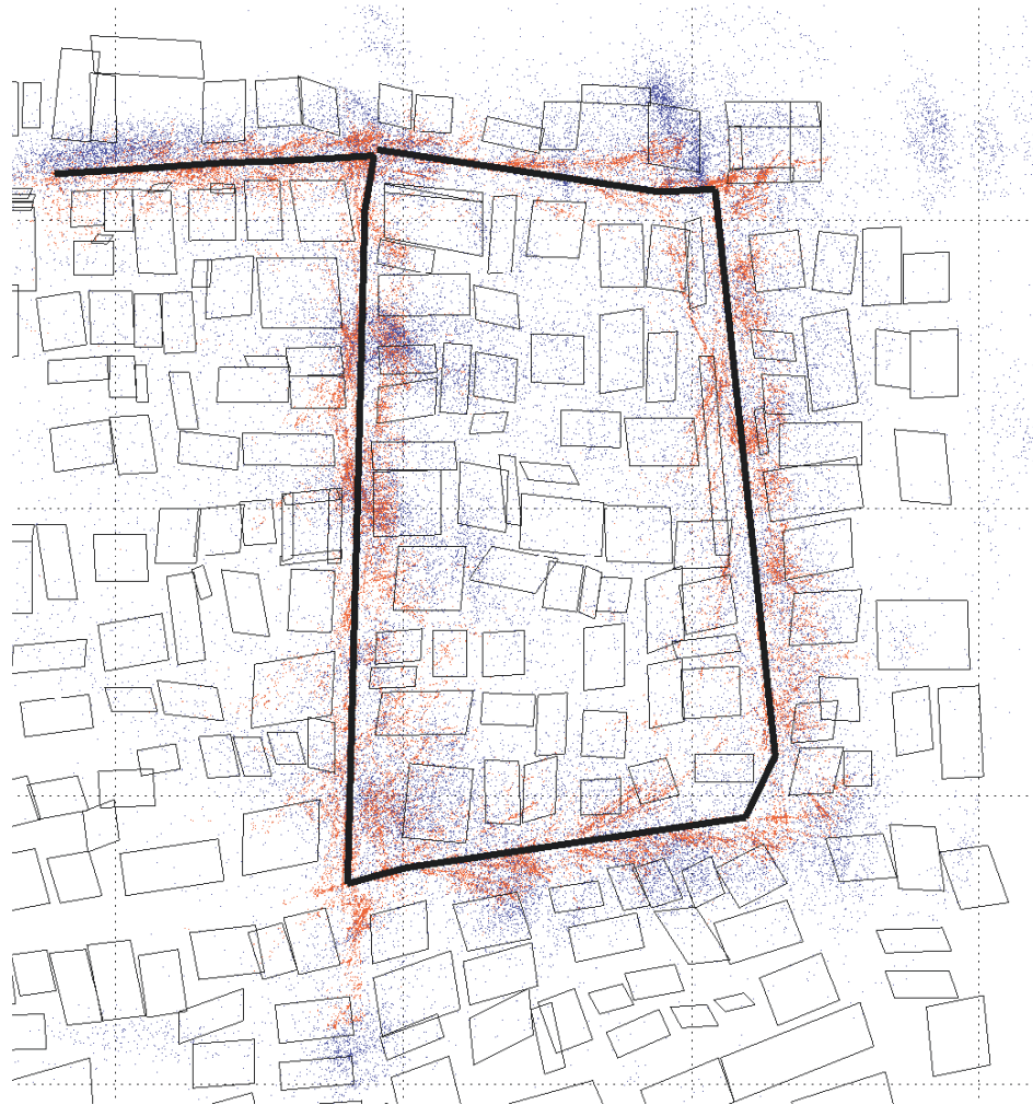
Fig. 5.73: Magnified view of Figure 5.72. The line indicates the trajectory of the MS. The red (darker) dots indicate the scatters seen by the BS, while the blue (lighter) ones the IOs at the mobile.
