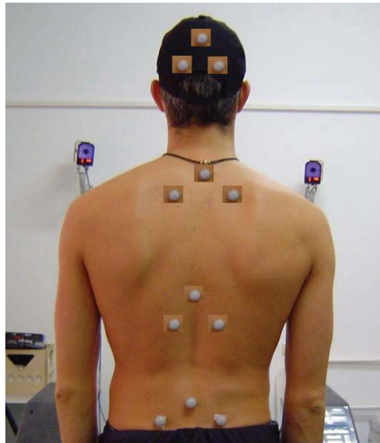
Figure 7- 2 Marker distribution. They represent the motion of pelvis, abdomen thorax and head.
