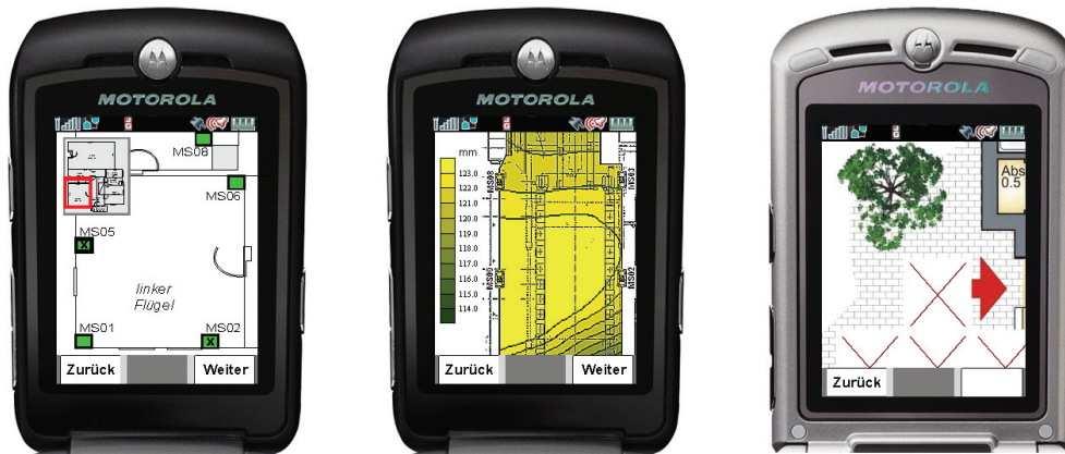
Figure 3: Possible operating surface for the MIDP application. Representation of a server-sided processed CAD file of the supervised object and overlapping with sprites for the eligible measuring points (on the left). Visualisation by contour plots (in the center) and a view with missing tiles marked as cross (on the right). The engineers can carry out by evaluation of the data an appraisal and initiate countermeasures in border-valued situations. To be able to analyze on site the topical data, the integration of mobile devices was necessary.
