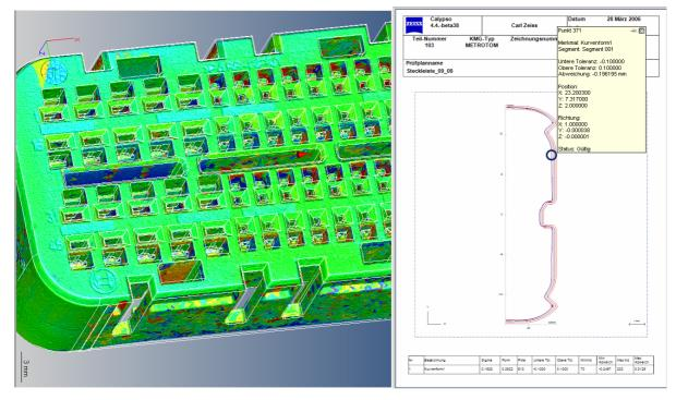
Once the surface points have been extracted from the volumetric data, CALYPSO offers many possibilities of visualizing the measurement results, such as color-coded model views or curve plots comparing nominal and actual surface positions.
