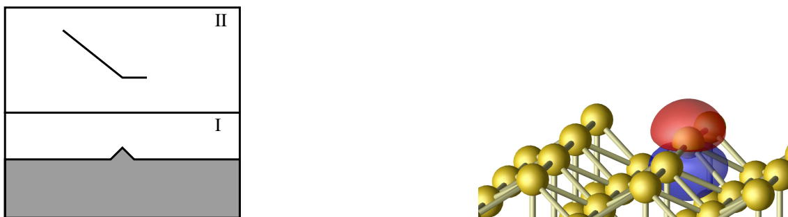
Figure 7.3: Left: Decomposition in subsystems I and II (see text). Right: Charge-density difference with regions of electron accumulation/depletion displayed in blue/red, isosurface value: \pm 0.02 e/\text{\AA}^3 , illustrating the dipole accompanying the structural changes in the substrate.
