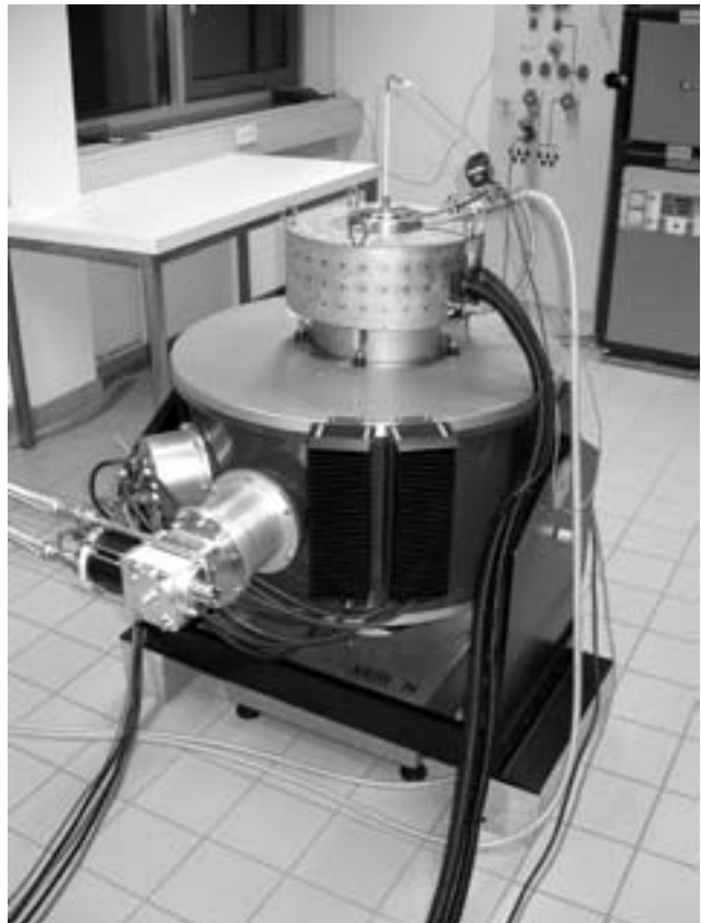
Fig. 1: Cryogen free 5T-DC-magnet with high temperature furnace.
