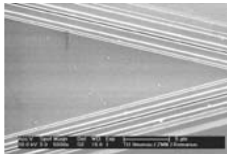
Fig. 2: SEM image of the V-pattern to locate the SiC nanostructures in by AFM.
