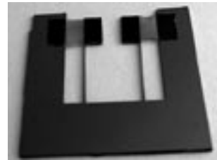
Fig. 5: Free standing elastomer membranes released by ASE
