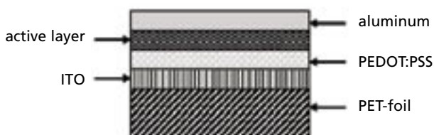
Fig. 1: Structure of the photovoltaic device.
