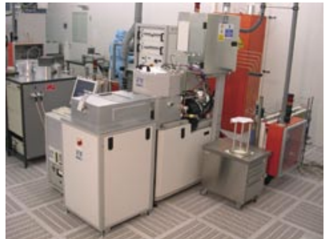
ICP-ASE dry etching process for silicon
