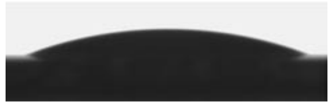
Fig. 2: Water droplet on hydrophilic oxidized AlGaN surface.
