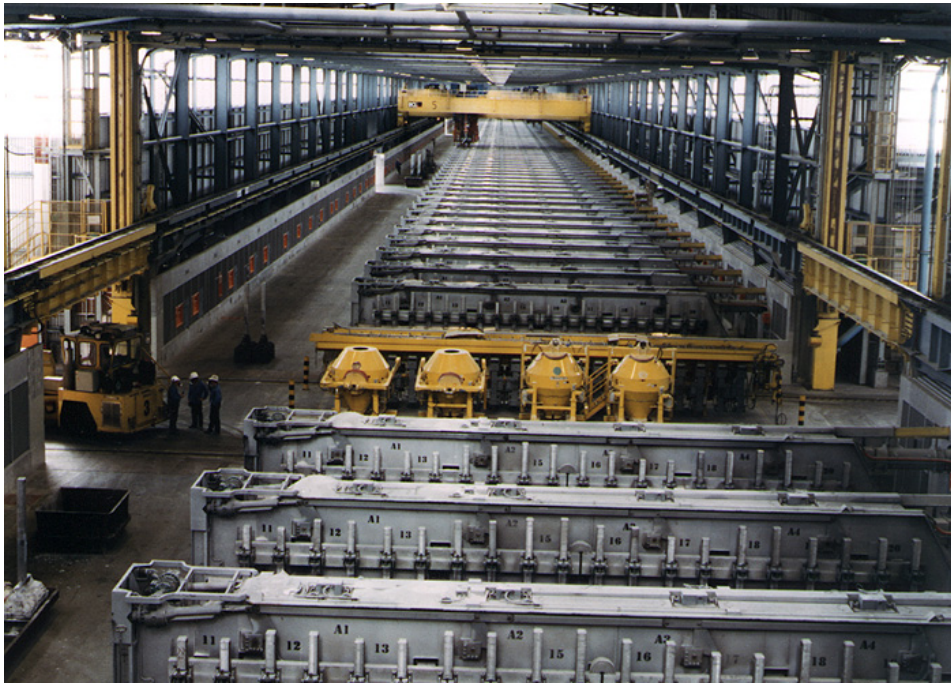
Figure 1.2: A reduction line (sometimes called a potline) at Boyne Smelters Limited, near Gladstone, Queensland, Australia. Comalco.
