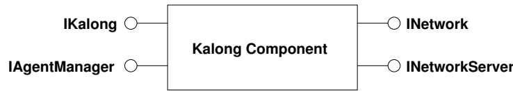
Figure 8.1.: The Kalong software component and its interfaces.
