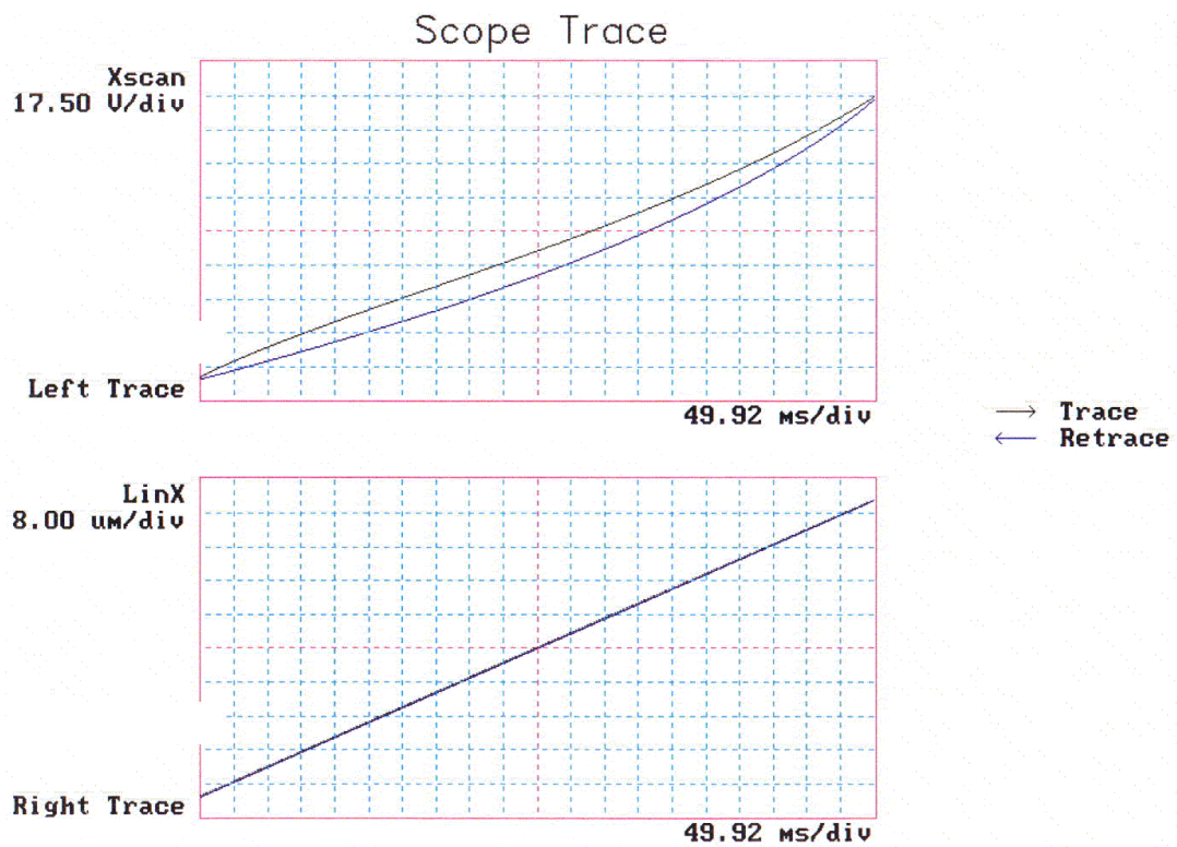
Figure 5.3 Linearity test in X direction with constant speed
