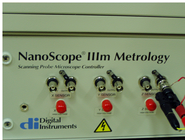
Figure 3.3 The modified controller of DI AFM
