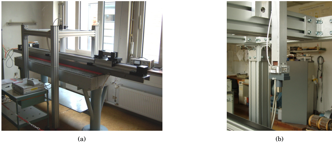
Figure 2.12: Improved version of the second experimental setup for LET [141]: (a) overview of the mechanical components; (b) detailed view on the multi-component force sensor and the attached cylindrical PM.
