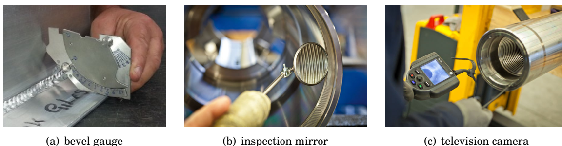
Figure 2.6: Examples of VT: (a) shape tolerance testing of welded component [4]; (b) and (c) visual quality inspection of an inside thread [69].
