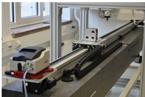
Figure 4.4: Experimental setup for experimental characterization of the linear guide using a long range multi-beam interferometer by SIOS Meßtechnik GmbH . The measurement reflector is placed on the slide for static and dynamic measurements of positioning deviation, pitch and yaw angle [109].
