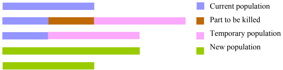
Figure 9: An evolution scheme using self-adaptive population control in a multi-population environment. The population size takes an unfixed value which is subjected to increase when the average fitness score in this population decrease.
