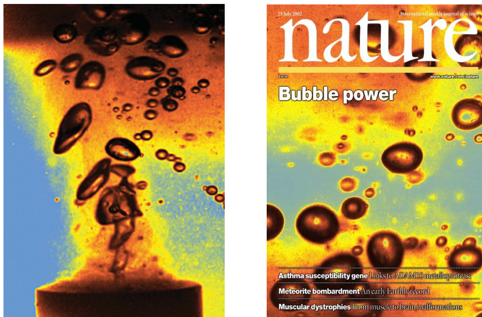
Picture 3 Cavitation bubbles: When a gas bubble in a liquid is excited by ultrasonic acoustic waves, it can emit short flashes of light suggestive of extreme temperatures inside the bubble. (Cover photo credit: K. S. Suslick and K. J. Kolbeck, Nature , 25 July 2002) [ http://www.scs.uiuc.edu/suslick/execsummsono.html ]
