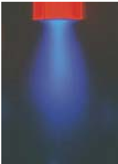
Picture 1 Sonochemistry: Sound waves can create high-energy bubbles in liquids. Intense heat and quick cooling of these bubbles speed up chemical reactions. [ www.aip.org/success/soundinvestment/ ]
