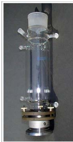
Figure 3-2 Ultrasonic transducer and a double-walled cylindrical glass reactor
