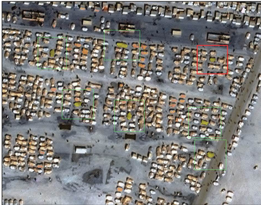
Figure 1.2. An example image analysis task where the aim could be to identify and characterise all structures. Seven tents were digitised and presented to a generic sample supervised segment generation method as reference segments.
