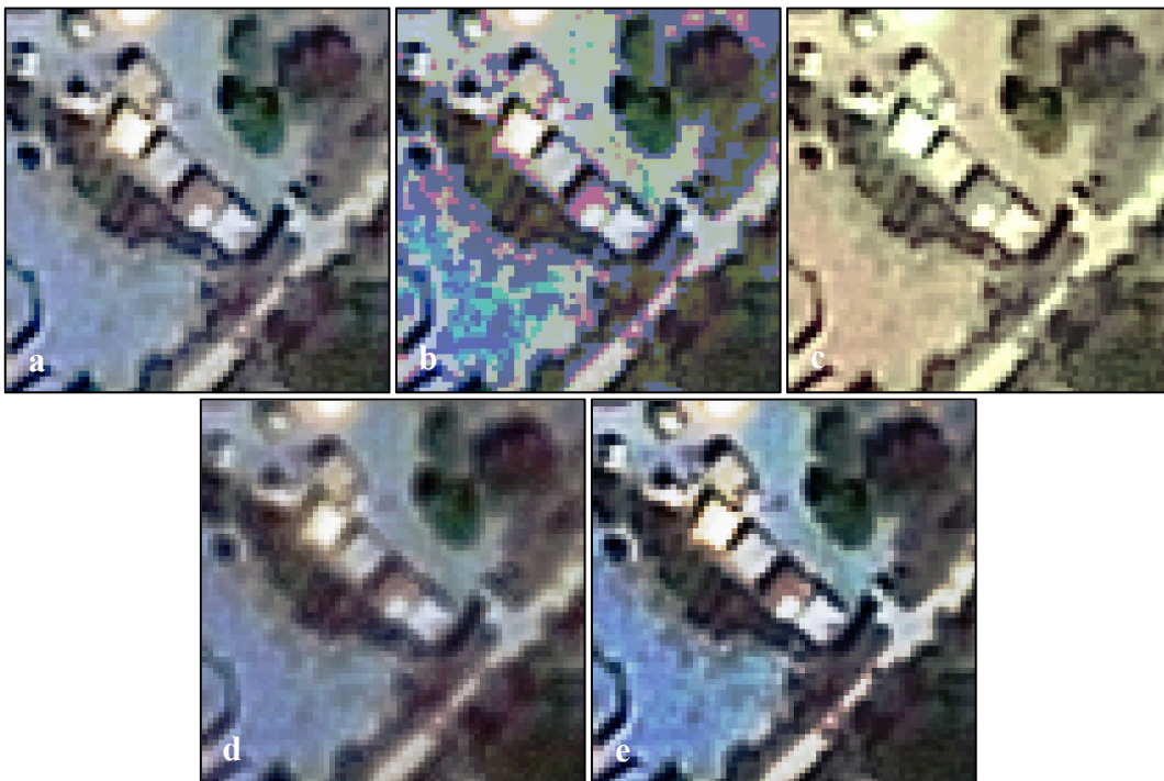
Figure 3.5. Output imagery from four data transformation functions tested in this work as part of a combined search space: (a) No Transformation, (b) Spectral Split, (c) Transformation Matrix, (d) Genetic Contrast, (e) Genetic Transform.
