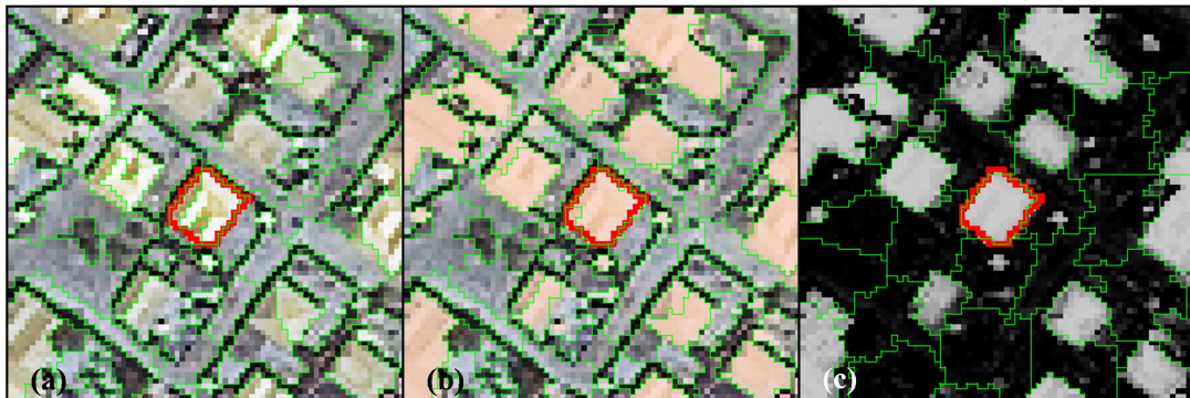
Figure 5.7. Segmented subsets, generated with the MS algorithm using the (a) original image, and a (b) Hybrid:CP image and segments generated with SLIC using a (c) probability image.
