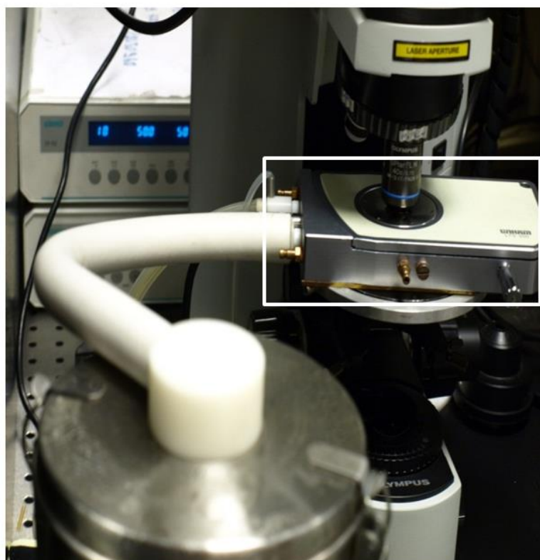
Figure 3.1 Experimental setup of the LTS420 heating/freezing stage, installed onto the Raman microscope setup.
