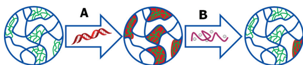
Figure 5. Schematic representation of the DNA uptake and release by the composite materials. (A) Uptake of fluorescently labeled DNA by the hydrogel component and (B) release of DNA by the addition of heparin.
