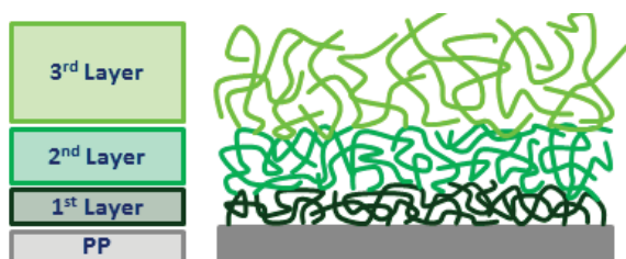
Figure 2: Schematically representation of water-swollen POx multi-layers.
