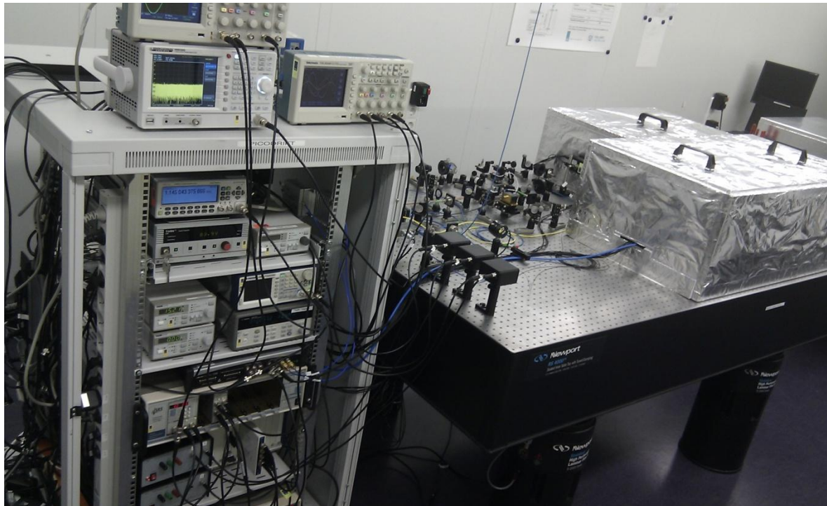
Figure 1: Overview of the Picodrift instrument. The control and measurement instrumentation is placed in and on top of the rack next to the optical table. The diode laser, several detectors, electro-optics modulator (EOM), acousto-optic modulators (AOMs), camera, and the required optical components for manipulation of the laser beam are positioned on top of the optical table. The ULE reference cavity (smaller box), and the Picodrift interferometer (larger box), are located inside two aluminium foil covered boxes providing additional thermal shielding.
