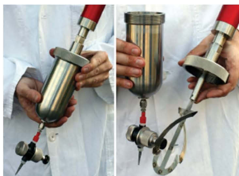
FIGURE 5 Fluid container equipped with overhead stirrer for storage of the formulations (PF and IF). [Color figure can be viewed in the online issue, which is available at wileyonlinelibrary.com .]
