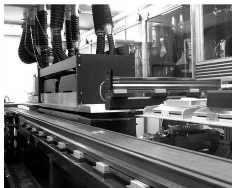
FIGURE 2 Detailed view of the high-throughput coating platform at Flamac.
