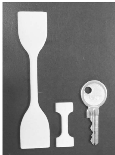
FIGURE 9 Conventional test specimen for physical characterization according to norm DIN 53504 S1 (left); microtensile specimen for the physical characterization according to norm ASTM D1708 (right).
