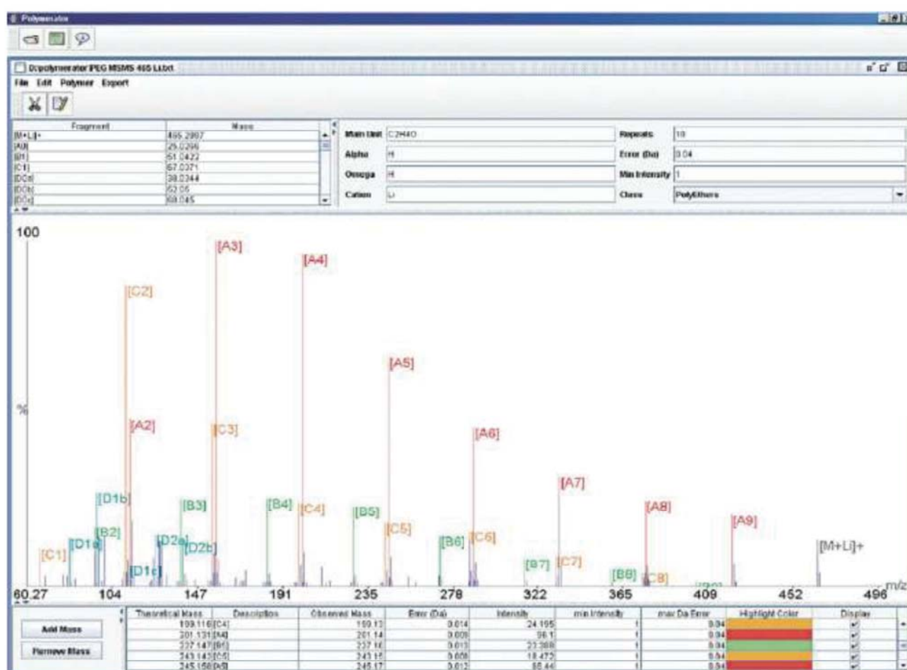
Figure 7 Screenshot of software with an annotated ESI-MS/MS spectrum from the lithiated decamer of PEG. Details of annotated fragment ions are displayed by the software in the table below the spectrum. Predicted fragment ions are also detailed above (left) of the spectrum. Reproduced from Ref. [83] with permission of the American Society for Mass Spectrometry.
