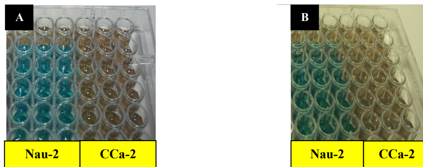
(Fig. 25) Color of the dye has changed with NAu-2 only and not with CCA-2 when both minerals were inocubated with S. commune (A), and with S. acidiscabies (B).
