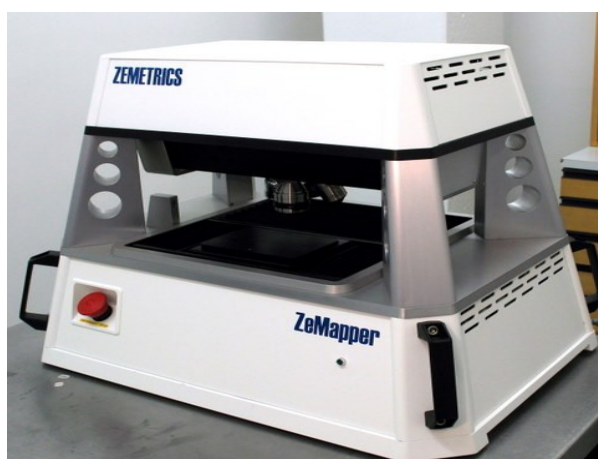
(Fig. 8) VSI device with a schematic diagram.
