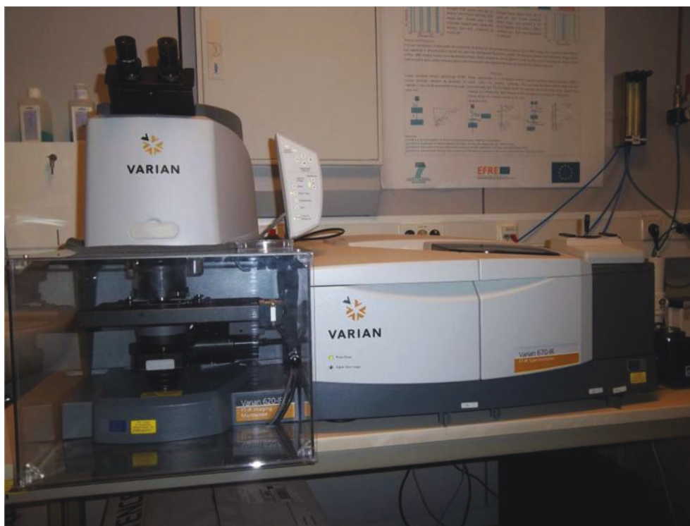
Fig. 3.11: Varian model 670, equipped with a microscope model 620, of a FTIR microscopic imaging.
