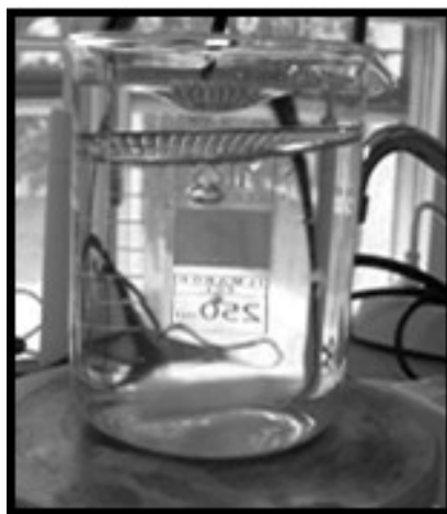
Fig. 55. Washing-test of glass surface covered by cellulose-4-[ N -methylammonium]butyrate chloride immersed in a water flow-bath.
