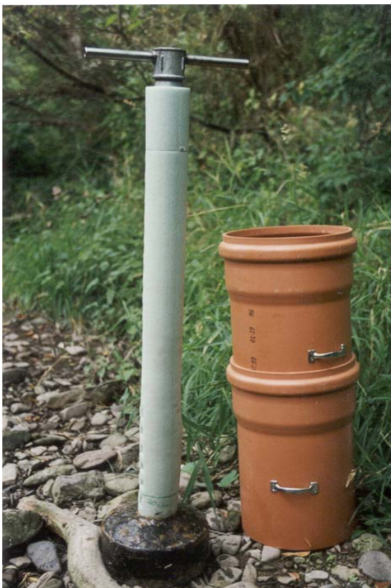
Figure 13: The Bottom-Sampler (left) and two stacked jackets (right).
