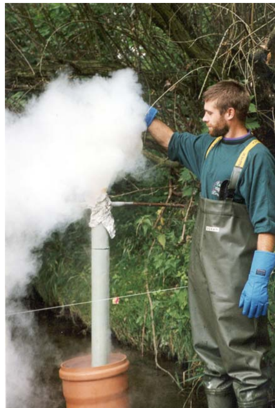
Figure 14: Freezing process during Bottom sampling: the liquid nitrogen is poured into the refrigerant pipe.
