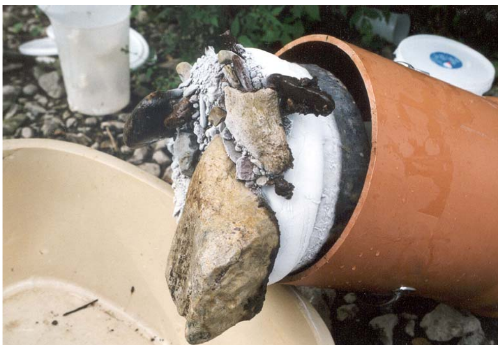
Figure 15: View at the ice-sediment mix disc attached at the Bottom-Sampler basis shortly after removal from stream.
