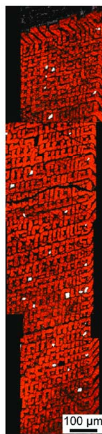
Figure 6. Deviating crystals (white) in a merger of OIM-scans within a dendrite of fresnoite cut perpendicular to the c -axis. The main orientation is marked orange.
