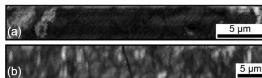
Fig. 4 Topmost segments of the IQ-maps of two OIM-scans performed with different step sizes on the unpolished surface of crystallised samples.
